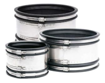
There are no spot-welds on the shear band having been replaced with fasteners using TOX <sup>®</sup> technology that enhances the corrosion resistance of the couplings. Couplings are secured in place using the screw 'jubilee' type fastener.
