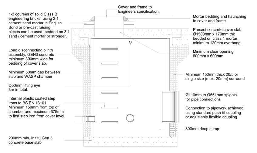
INSTALLATION DETAIL WASP05350 Series Prefabricated Catchpit Chamber Ø1500 up to 2.5m deep chamber By SEL Environmental Tel: 01254 589987
