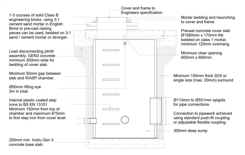
INSTALLATION DETAIL WASP05250 Series Prefabricated Catchpit Chamber Ø1200 up to 2.5m deep chamber By SEL Environmental Tel: 01254 589987
