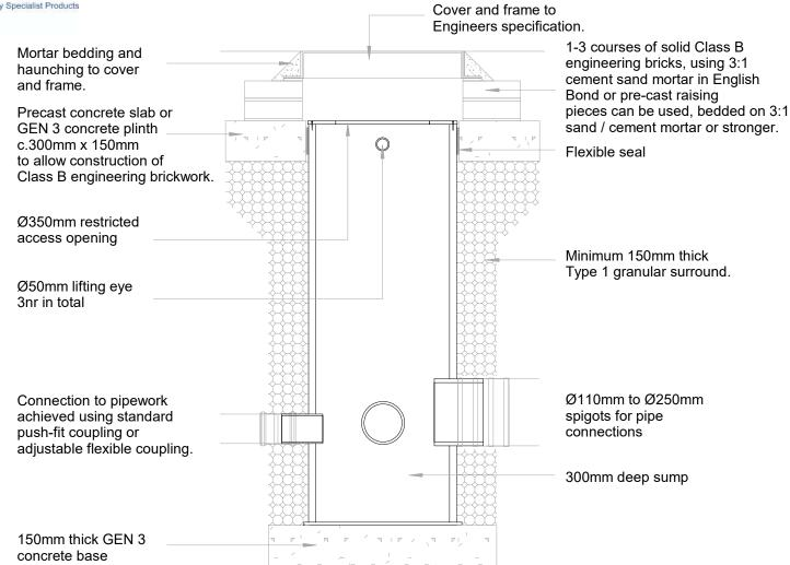
INSTALLATION DETAIL WASP05050 Series Prefabricated Catchpit Chamber Ø500 up to 2.5m deep chamber By SEL Environmental Tel: 01254 589987
