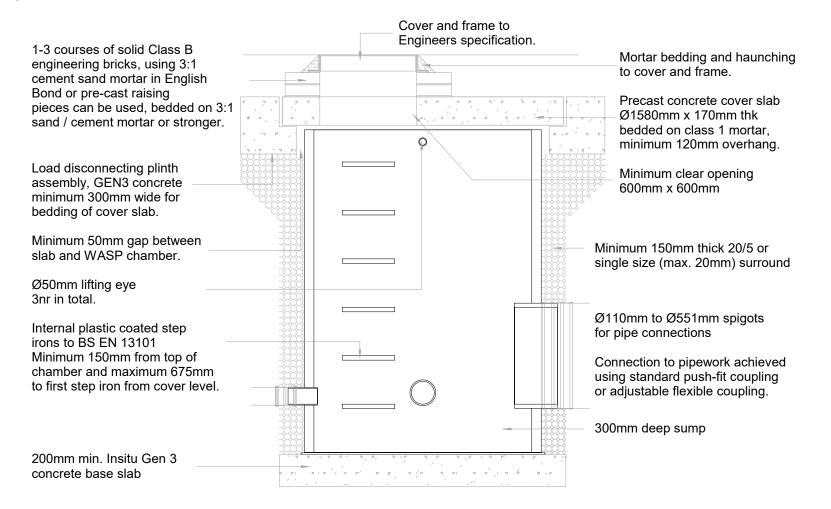
INSTALLATION DETAIL WASP05300 Series Prefabricated Catchpit Chamber Ø1350 up to 2.5m deep chamber By SEL Environmental Tel: 01254 589987
