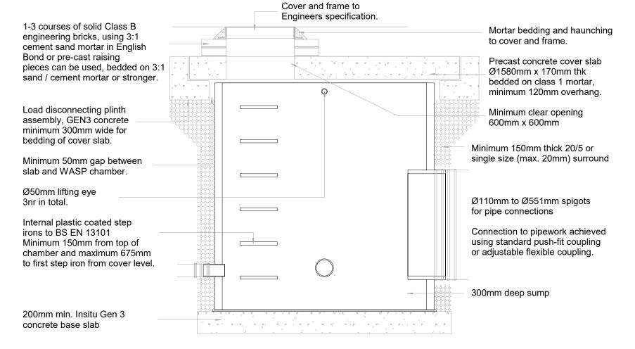
INSTALLATION DETAIL WASP05400 Series Prefabricated Catchpit Chamber Ø1800 up to 2.5m deep chamber By SEL Environmental Tel: 01254 589987
