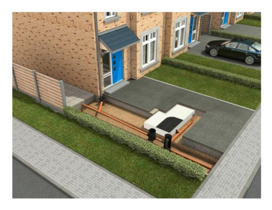
Each chamber has a 200mm deep sump to accommodate the deposition of any suspended solids remaining in the runoff which has passed through RWP Filter Chambers positioned at the base of all the downpipes.
