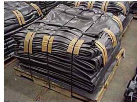
Prefabricated liner ready for dispatch
