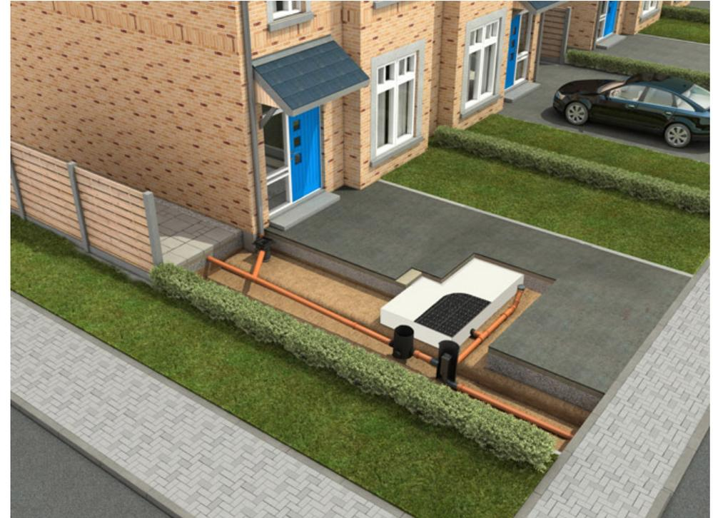
Each chamber has a 200mm deep sump to accommodate the deposition of any suspended solids remaining in the runoff which has passed through RWP Filter Chambers positioned at the base of all the downpipes.
