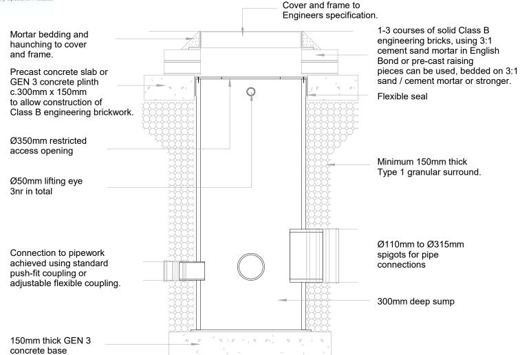
INSTALLATION DETAIL WASP05100 Series Prefabricated Catchpit Chamber Ø600 up to 2.5m deep chamber By SEL Environmental Tel: 01254 589987
