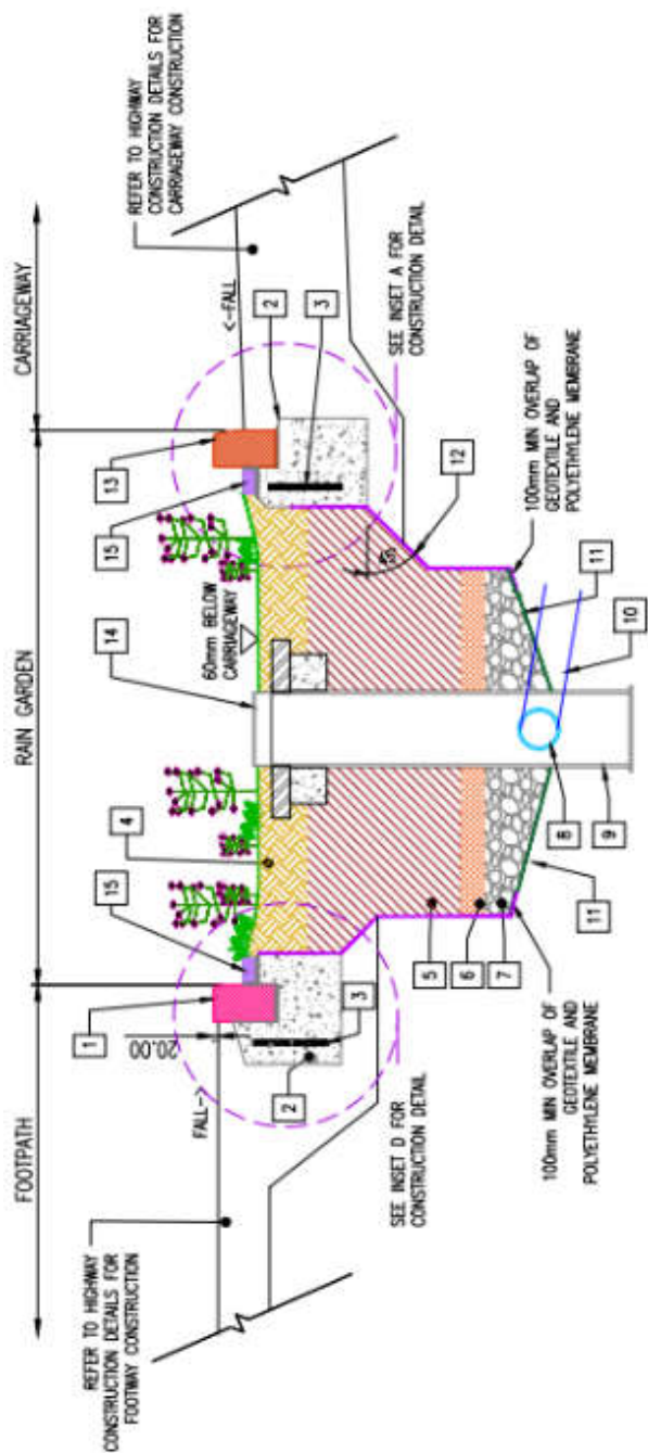
TYPICAL RAIN GARDEN SECTION 'GULLY LOCATED CENTRALLY' Section A-A
